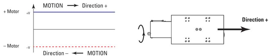
In the above drawings, + Motor signal is referred to – Motor signal.
