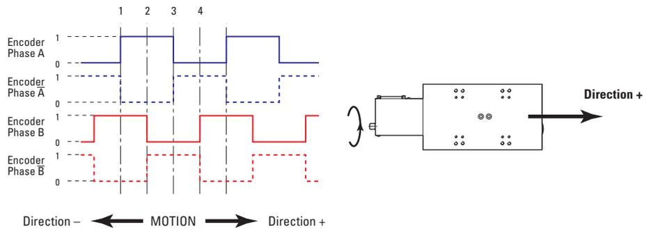
The incremental sensor consists of an optical scale and an encoder head. When the carriage moves, the encoder head generates square signals in quadrature and sends to pins #19, #20, #23 and #24 of the SUB-D25 connector.
